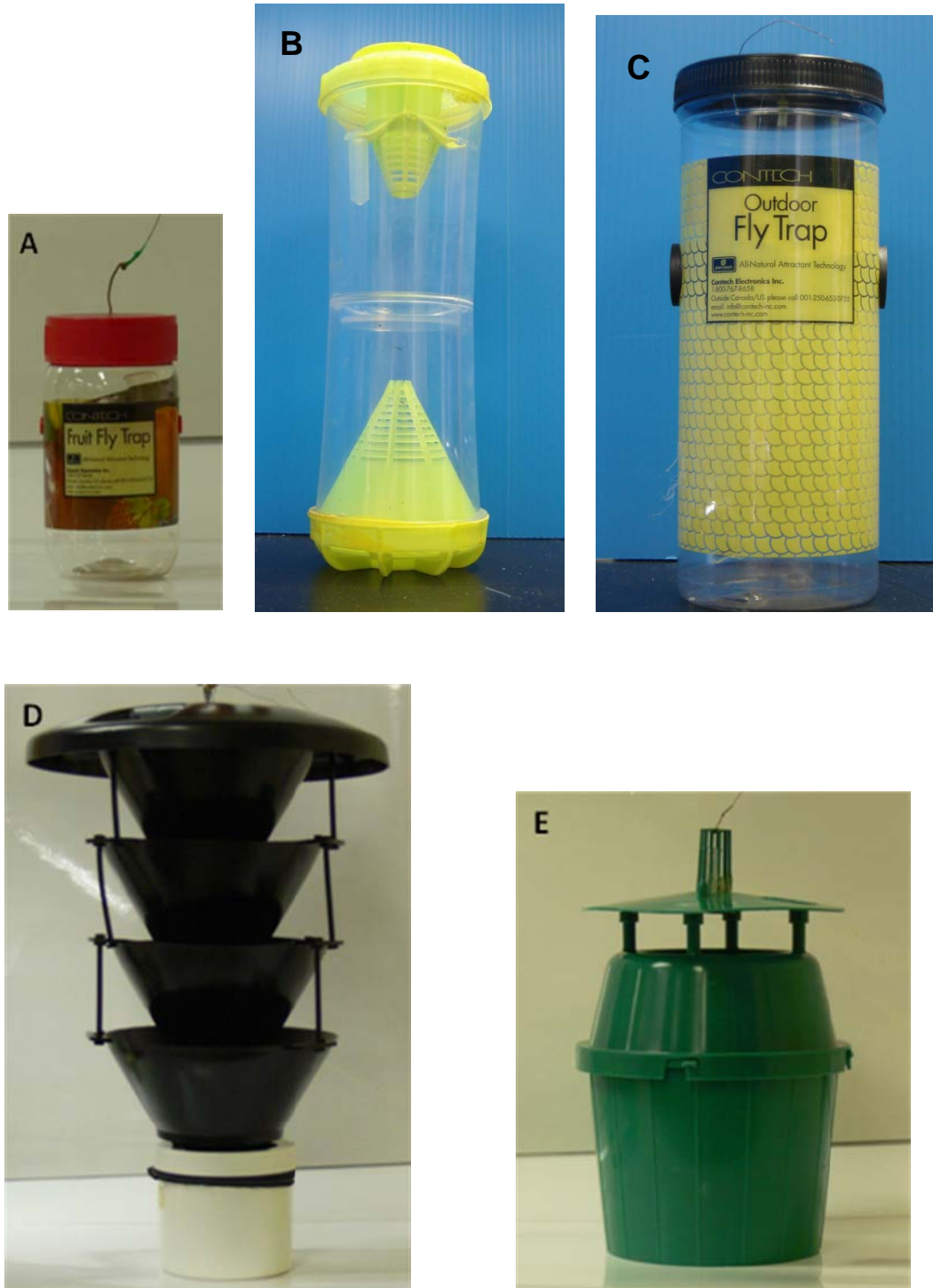
Figure 5. Candidate soap and water traps that were evaluated for their ability to capture Harmonia axyridis . The follow traps were tested: (A) Contech® Fruit Fly trap; (B) Rescue!® WHY trap; (C) Contech® Outdoor Fly trap; (D) Lindgren funnel trap; (E) Universal trap.
