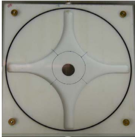
Figure 1. Overhead view of the four arm olfactometer. The arena was divided into five areas, one central area (8 cm diameter) and four other areas corresponding to each arm of the olfactometer. Boundaries were superimposed onto the arena using a video monitor. Air was simultaneously pushed into the arena through 4 inflows and drawn through the central hole in the floor of the arena. Test compounds were introduced into one arm while the other three arms were controls. External dimensions: 32 × 32 × 2.5 cm. Internal height of arena: 1.8 cm. Central hole in the floor: 3.2 cm diameter.
